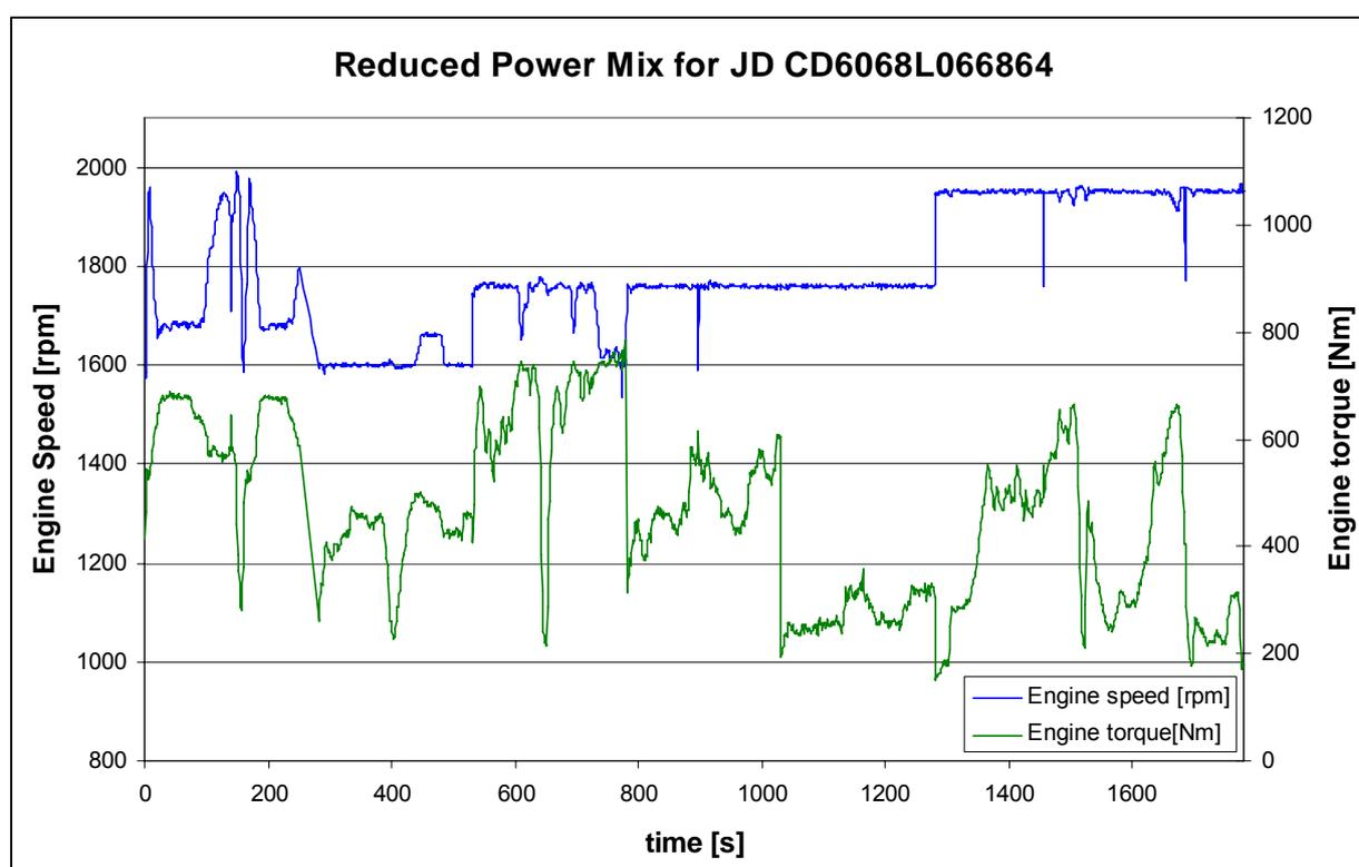
Fig. 8 Engine speed and torque over time for the CD6068L066864 at the LVK-TUM test stand
