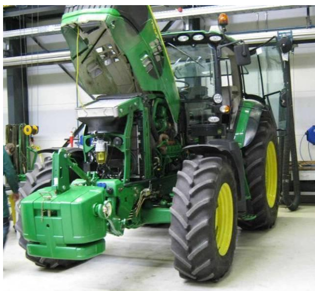
Figure 1: JD tractor, converted to Euro stage 3B and 4
