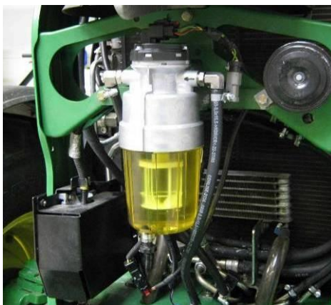
Figure 6: pre pressurization pump with pre fuel filter, mounted in front of the engine air cooler (concerted stage 3B and 4 tractor)
