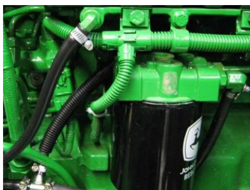
Figure 7: main fuel filter, mounted left side of the tractor
