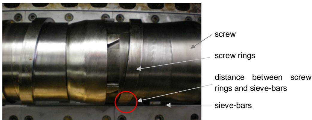
Picture 6: Screw of oil mill for corn germ processing<sup>32</sup>
